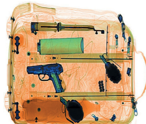
Improved classification of materials: orange – organic, blue – metals, green – mixed materials
