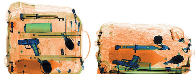
Improved classification of materials: orange – organic, blue – metals, green – mixed materials
