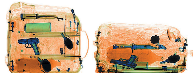
Improved classification of materials: orange – organic, blue – metals, green – mixed materials
